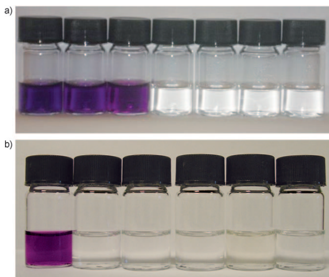
Figure 6. a) Degassed 1 \times 10^{-4} M solutions of host 2 in the presence of the TBA salts (1 equiv) of the following anions (from left to right): succinate, malonate, acetate, chloride, bromide, nitrate and perchlorate. b) Degassed 1 \times 10^{-4} M solutions of hosts 6 in the presence of the TBA salts (1 equiv) of the following anions (from left to right): acetate, malonate, chloride, bromide, iodide and nitrate.
